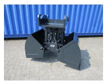
Multi-use grab for a wide range of applications for handling different materials such as demolition, sorting scrap, loading and sorting and recycled materials.
