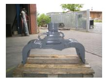
Multi-use grab for a wide range of set of handling different materials such as demolition, sorting scrap, loading and sorting and recycled materials.
