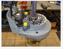
The DWP-15-2 slewing gear has been designed for use on hydraulic attachments for hydraulic excavators, as well as for mobile and stationary handling machines. The DWP-15-2 takes over three functions for the operation of the attachment:
