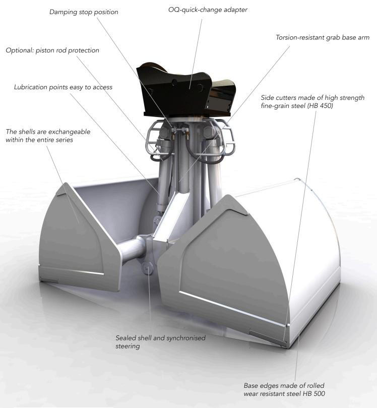
Optimized grabs for the transfer of bulk materials such as gravel, sand, pebbles, grain, feed, fertilizer, ore, coal, etc.
