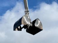
Optimised grab for running light goods such as light granulate, grain, feed, fertilizer.
