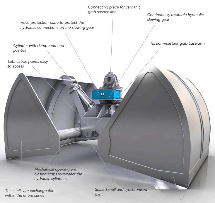
Side and base edges made of high strength fine-grain steel (HB 450) and with reinforced weld-on profiles (HB 500)
