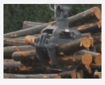
Handling grab for logs and round timber. Due to the shape of the tines, TG2 wood grabs can easily pick up one or more logs of different diameter from the ground, a stack or HGV and confidently hold and handle them.
